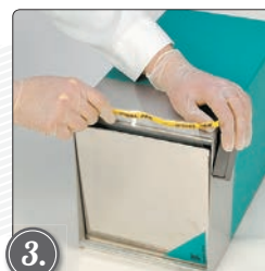
3. Close door, paddles start automatically or with switch, door holds the bag in place.
