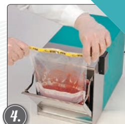
4. When time has elapsed, open door, remove bag, and test sample.
