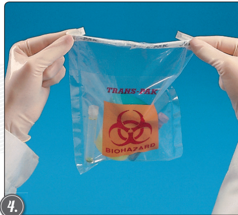
4. Bend wire ends back to seal bag.
