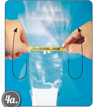
4a. Hold bag by the wire ends and whirl three times for the tightest seal.
