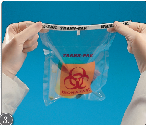
3. Fold top of the bag down three times to close.
