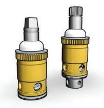
WaterSaver faucets utilize an interchangeable unit or cartridge that is standardized across the product line. The unit contains all working components of the water faucet or valve. There are no moving parts in the faucet or valve body itself to wear out. As a result, WaterSaver water fittings are virtually everlasting.
