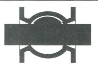
In the full-open position, the plug is rotated out of the main fluid stream as shown. This allows for high capacity flow through the valve.
