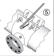
**Step 6** • Bolt tapping valve to flange. The inside of the flange accepts the tapping valve locator. The flange gasket is provided
