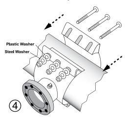
Step 5 • Install washers, (plastic first, then steel) and nuts. Tighten uniformly to a minimum 90 - 100 ft-lbs. torque. The gap between sleeve halves should be equal on both sides when the nuts are fully torqued.
