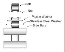
**Note:** On 4" nominal SSTIII's install sleeve bolts with the bolt heads facing the flange for more flange bolt clearance.
