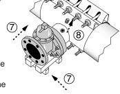
the table (below), whichever is less. If assembly leaks, check bolts to be sure the nuts have been torqued to the recommended torque value and then retest assembly.
