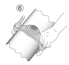
**Step 7** • In 15 - 20 ft-lbs. increments, tighten nuts to 30 - 35 ft-lbs. Keep bolts tight to the body. Use a wrench with at least a 12 inch handle.
