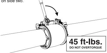
**Step 7** • Confirm proper installation by pressurizing the line and checking for leaks.
