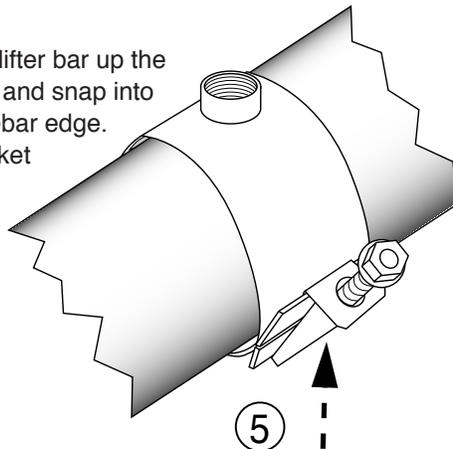
**Step 6** • Tighten all nuts evenly in 20 ft-lbs. increments. Use a wrench with at least a 12 inch handle.
