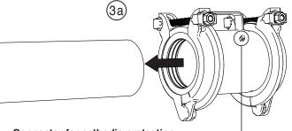
Connector for cathodic protection.
