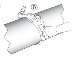
**Step 7** • Tighten all nuts evenly in 15-20 ft-lbs. increments. Keep bolts tight to the body. Use a wrench with at least a 12 inch handle.
