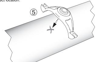
Step 6 • Install strap(s) on saddle body, and tighten finger tight. Make sure the gasket has seated itself flat onto the pipe face.
