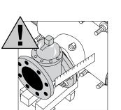
NOTE: Be sure to measure the gap between flange faces all the way around the valve, to ensure valve flange and tapping sleeve flange are parallel.
