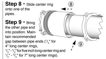
Step 10 • The center ring should be centered such that the space between the OD of the pipe and the ID of the center ring is even all around the pipe. Slide gaskets into position with the beveled edge engaging the flared end of the center
