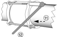
Step 12 · Insert bolts into end rings and
