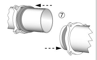
Note: Flexible Couplings do not provide protection against possible pullout of pipe ends in unrestrained conditions.
