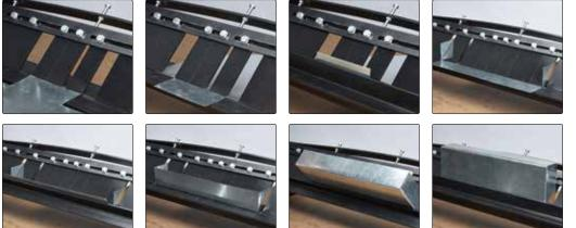
When forming pans and boxes, remove & position finger plates as needed to span widths.
