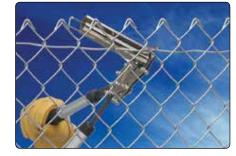
Commercial grade Hog Ring Pliers with Magazine installs 9-Ga. (3.8 mm) collated aluminum rings or exclusive 9-Ga. (3.8 mm) collated steel rings. Easily secures 7-Ga. (4.5 mm) wire to 9-Ga. (3.8 mm) chain link fence.
