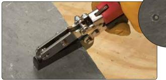
The NSP1EV Slate Punch produces a clean, recessed nail hole in 4 – 8 mm natural roofing slate. A big 2-1/2-inch (63 mm) throat depth allows convenient placement of the punch tip on the flat, unfinished side of the slate to create a desirable nail hole recess on the natural finished side as it punches through. Hardened all-steel construction with rust-resistant nickel plate and black oxide finishes ensures long service. The tool steel punch component is also replaceable.
