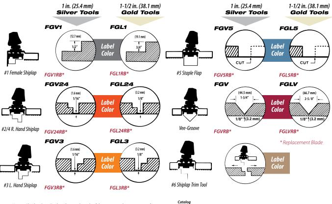
Use #6 Shiplap Trim Tool to shorten length of duct section, by measuring from outside edge of material to be scrapped. Avail. for 1 in. (25.4 mm) board only.
