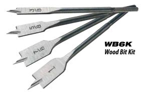
Unique designed ground points and cutting edges drill faster, cleaner holes, using less power than standard spade type bits. Cut straight or angled holes in soft and hard woods, plus formica, plaster, chipboard, foam core material, many non-metallic building sidings and foam insulation. Made of one-piece special heat treated tool grade steel.
