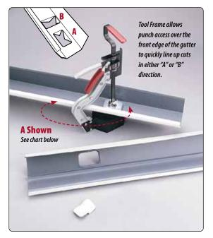
Gutter Size Reference:Following Gutter Sizes Do Not Fit "B" Direction:4K Gutter -2 x 3, 2 x 3 X-Style, 3 x 4, 3 x 4 X-Style5K Gutter -3 x 4, 3 x 4 X-Style6K Gutter -3 x 4, 3 x 4 X-Style
