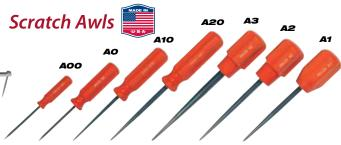
Use to scribe lines on metal, plastic and a variety of other materials. Pierce holes in wood, plastic, leather, - even light gauge metal. Blades are high carbon, alloy tool steel fully polished to resist rust. Blade tapers to a fine point and may be resharpened many times. Easy-to-spot orange handles are shock and shatter resistant. Shallow fluted handles with large end bearing surface provide a sure, comfortable grip. User has choice of large diameter or regular grip handles.
