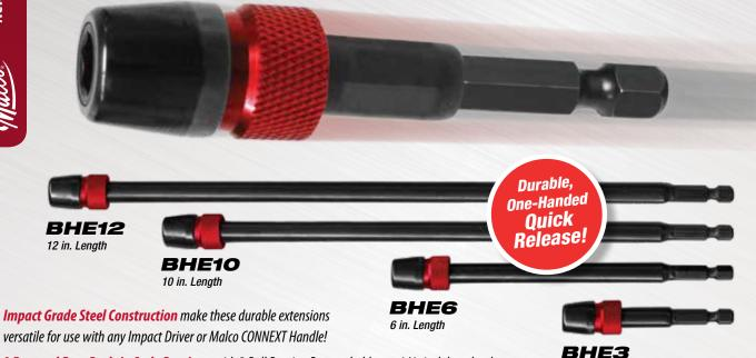
**A Fast and Easy Push-in Style Receiver**, with 3 Ball Bearing Detents holds any 1/4 -inch hex shank power groove or insert bit securely. Retract the collar only when removing bit.
