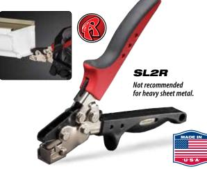
Slide adjustment for throat depth allows settings from 1/4 to 5/8 in. (6 to 16 mm) depth. Easy one-hand operation. Ideal for crimping gutter end caps in place. Also creates locking tabs in light sheet metals for joining metal sheets or inserting into rolled edge of utility trim. Formed metal cutting jaws and handles are made of hardened stampings. Rust resistant nickel plate and black oxide finishes ensure long service life.
