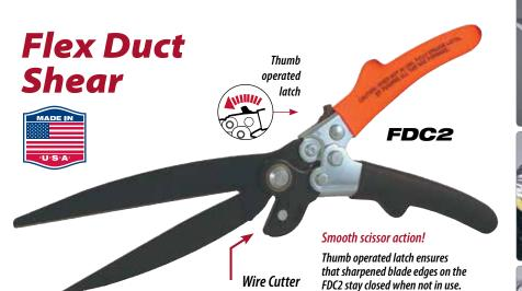
Cuts insulated flexible round duct and also cuts the duct liner's wire rib coil. Pointed bottom blade easily pierces duct to start cut. Heavy duty wire cutter is located away from scissor blades. Thumb operated latch ensures that sharpened blade edges stay closed when not in use.
