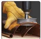
This Combination Hole Saw Style Arbor and High Speed Steel Pilot Drill is specifically designed for use with Malco Gutter Outlet Saws. One universal threaded arbor quickly installs on any size Gutter Saw. The pilot drill bit projects only 7/16 in (11 mm) out of the shallow gutter saw cup to ensure controlled, safe engagement of saw teeth for hole cuts in K-style and half round gutter. A tapered compression spring collar on the drill bit automatically ejects the metal slug.
