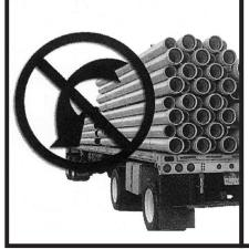
DO UNLOAD WITH FORKS THAT EXTEND TO SUPPORT ALL OF THE PIPE IN THE BUNDLE.
