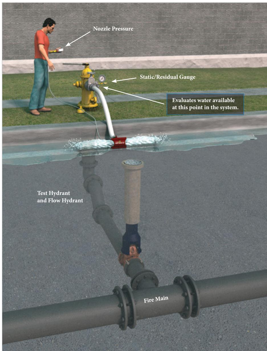
5. Slowly close gate valve, then close the hydrant. Remove test equipment from hydrant. Replace and tighten cap. If the hydrant is a dry barrel type, note that water drains properly from the hydrant. Remove Remote Reader and gauge from the Pitotless Nozzle.
