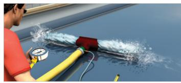
The Little Hose Monster and Pitotless Nozzle in a rooftop standpipe test.
