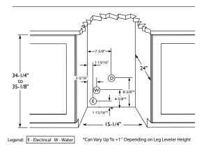
CLR2160 Stainless, Black, White and Overlay Models \* Add 3/4" to depth for drain line clearance
