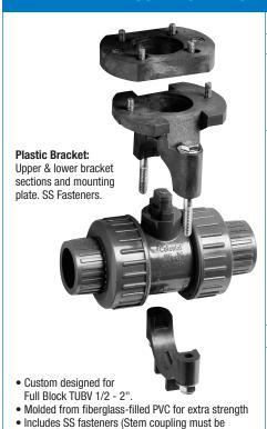
Can be retro-fitted to an installed Full Block TUBV
