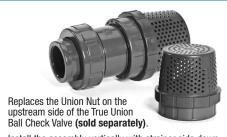
Install the assembly vertically with strainer side down. Prevents debris from entering the fluid stream of a suction pipeline. Valve opens when suction is activated. Ball then seats to close the valve when suction is not present.
