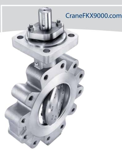
Torque-Seating: Unlike position-seated ball, butterfly or plug valves, the torque-seated Crane®FKX 9000 selfadjusts to evenly distribute seal compression. A "floating" seal ring and wide seal ring supporting gasket yield a BETTER SEAL to eliminate binding and to enhance performance.
