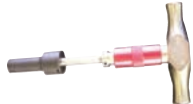
Torque Wrench Non-adjustable torque wrench factory set to 60 inch pounds. Accommodates both 5/16 and 3/8 inch fasteners.
