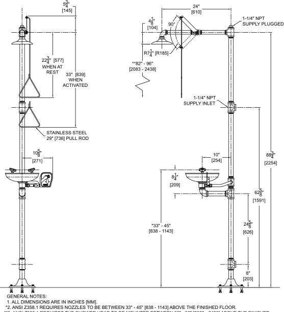
\*\*3. ANSI Z358.1 REQUIRES THE SHOWER HEAD TO BE MOUNTED BETWEEN 82" - 96" [2083 - 2438] ABOVE THE FINISHED FLOOR WITH A 16" [406] MINIMUM RADIUS UNOBSTRUCTED.
