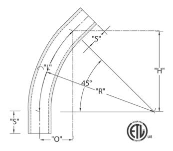
CANTEX 45-Degree Plain End Schedule 40 Special Radius Elbows are used to change the direction of a conduit run by 45 degrees when special radiuses are needed.
