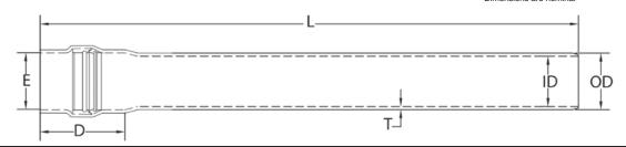
In a league of its own, CAN>GRIP delivers the easiest and fastest installation of any horizontal directional drilling conduit system available. The internal gripper locking-mechanism does all the work, so CAN>GRIP sections connect in one fast step! Just hit the plain end of the CAN>GRIP length into the belled-end until it is fully inserted and secure. No cement or external locking-mechanisms are needed! The unique belled end contains a patented Reiber Gasket to maintain a watertight system.
