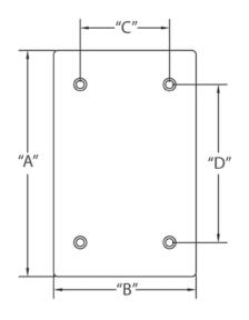
CANTEX 5133362 is a 1-Gang Weatherproof Blank Cover designed for use with exposed weatherproof boxes.
