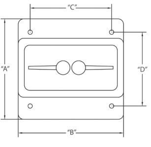
CANTEX 5133331 is a 2-Gang Weatherproof Toggle Switch Cover designed for use with exposed weatherproof boxes.
