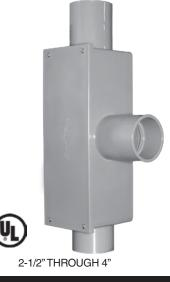
Conduit Body Type LR provides pull, splice, and tap access for conductors in a conduit system along with a change in direction. Type LR Conduit Bodies are used to make a 90-degree turn in a conduit run with one opening on top and one opening exiting the right side of the cover.
