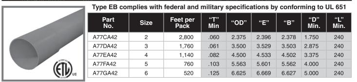
EB-20 PVC Utility Duct is designed for the power and communication industry to protect underground cables and raceways. It is designed to be used in concrete encased burial applications.
