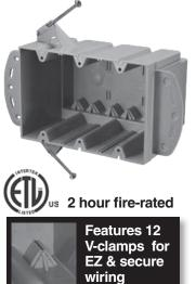
EZ74TNZ is a 74 cu. in., deep, 3-gang switch and outlet box for residential or light commercial new construction (new work) installations with molded brackets for steel stud mounting and screw-nails for EZ installation on aluminum, light to medium grade steel or wood studs. The screw-nail's sharp point, slotted head and threaded body allow for installation with a power screwdriver with no need for pre-drilling.
