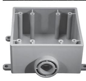
Exposed Boxes Type FSE are designed for use in indoor and outdoor locations where the boxes are exposed and subject to environmental conditions. Type FSE is intended for conduit termination with one conduit hub and no outlet.
