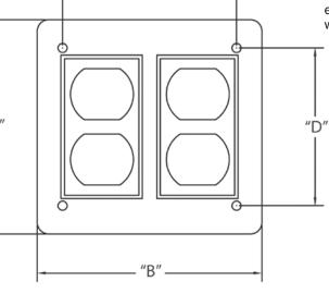
CANTEX 5133347 is a 2-Gang Weatherproof Double Duplex Cover designed for use with exposed weatherproof boxes.
