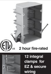
EZ44TN is a 44 cu. in., 3-gang, nail-on, electrical switch and outlet box for residential or light commercial new construction (new work) electrical installations. It features 12 wire clamps and enhanced angled nails for easy installation.
