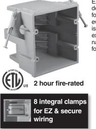
EZ35DN-HW is a 2-gang 35 cu. in. heavy wall residential EZ BOX that is ideal for new work applications for residential and light commercial projects where an even more durable box is preferred. The harder shell is designed to resist flexing and hold its shape in extreme conditions. It also features enhanced angled nails for easy mounting between studs 8 wire clamps for EZ and secure wiring.
