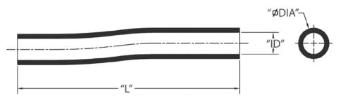
Conduit offset is a plain end section of conduit formed to go around obstacles or compensate for centerline differences in two conduit runs.
