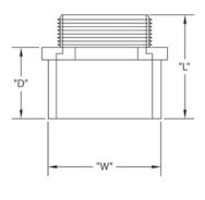
Male Terminal Adapters are connectors used to transition from a spigot end PVC conduit to a threaded metal or PVC plastic female bell end. Male Terminal Adapters can also be used to connect PVC conduit to a box or other threaded body with use of a lock nut. The fittings consist of one solvent weld female end and one threaded male end. Both ends will fit the same diameter conduit.
