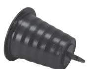
Poly Plugs with Pulling Eyes are designed for the temporary sealing of conduit to protect the duct from the effects of weather, job site debris, and animal damage. The molded in pull-eye is used to secure excess pulling rope within conduit.
