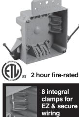
EZ18XN is an 18 cu. in., 4" square, PVC box for residential or light commercial new construction (new work) electrical installations with a molded flange and enhanced angled nails for EZ mounting options. 4" square boxes provide maximum volume for multiple conductors and connectors that often run in two or more directions. Great for walls or ceilings for fixtures, switches or receptacles. CANTEX 4" square boxes are often used with solid PVC blank covers like CANTEX EZXKL.
