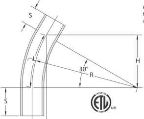
CANTEX 30-Degree Plain End Schedule 40 Special Radius Elbows are used to change the direction of a conduit run by 30 degrees when special radiuses are needed.
