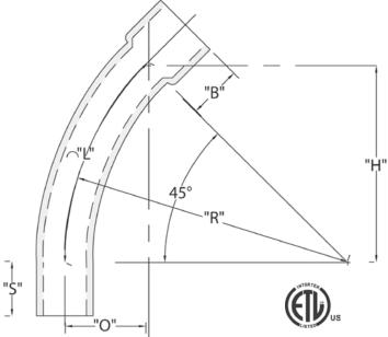
CANTEX Belled End Schedule 80 45-Degree Special Radius Elbows are used to change the direction of a conduit run by 45 degrees when special radiuses are needed.
