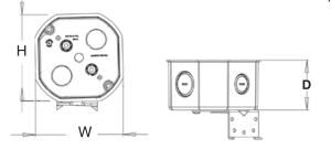
CANTEX EN20CB is a 20 cu. in. Octagon ENT Ceiling Box with an L-Bracket. It is for residential and light commercial ceiling fixture applications. It features an L-bracket for EZ and secure installation and 6 knockouts for multiple wiring options.
