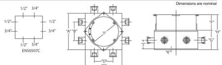
CANTEX ENS0507C is a 55.5 cu. in. ENT Slab Box with 1/2 & 3/4 inch Snap-In Connectors designed for use with electrical nonmetallic tubing (ENT) and standard electrical devices and switches in residential and light commercial applications.
