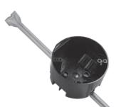
EZ20CH EZ BOX is a 20 cu. in., new work (new construction) ceiling box with an attached bar hanger for adjustable, support between ceiling joists. EZ20CH is for residential and light commercial ceiling applications. EZ20CH features 6 wire clamps and an adjustable bar hanger that adjusts from 14" to 18" for added support and installation options. The EZ20CHL hanger bar adjusts from 18 in. to 24 in.
