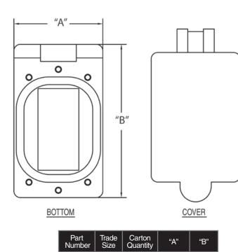
CANTEX 5133348 is a 1-Gang Weatherproof GFI Receptacle Cover designed for use with exposed weatherproof boxes.
