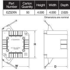
EZ BOX® Shallow Bracketed New Work Nail-on Switch & Outlet Box
