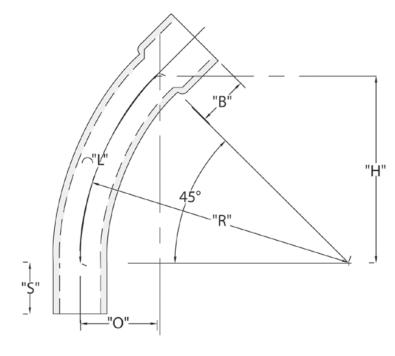
DB-60 Special Radius Bell End 45 Degree Elbows are used to change the direction of a conduit run by 45 degrees.
