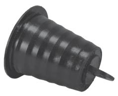
Poly Plugs with Pulling Eyes are designed for the temporary sealing of conduit to protect the duct from the effects of weather, job site debris, and animal damage. The molded pull-eye is used to secure excess pulling rope within conduit.
