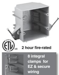
EZ32DN EZ BOX is a 32 cu. in., 2-gang, nail-on, electrical switch and outlet box for residential or light commercial new construction (new work) electrical installations. It features 8 wire clamps and enhanced angled nails for EZ installation.
