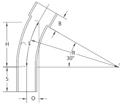
DB-120 Special Radius Bell End 30-Degree Elbows are used to change the direction of a conduit run by 30 degrees.
