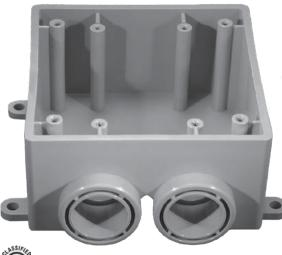
Exposed Boxes Type FSS designed for use in indoor and outdoor locations where boxes are exposed and subject to environmental conditions. Type FSS is intended for conduit termination with two conduit hubs on one end and no outlet.
