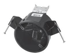
EZ25CF-HW EZ BOX ceiling fan box is a nail-on, heavy duty ceiling fan box for new work (construction) applications for residential and light commercial projects. It features a harder shell that will not break or change shape in extreme conditions. It also features an attached metal nail-on L-bracket for easy installation and added support. CANTEX ceiling boxes are constructed with durable polycarbonate for added resilience.
