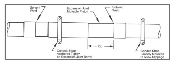
The correct piston setting, Dp, can be determined for any installation temperature by using the following equation:
