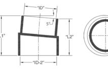
Schedule 40 5-Degree Couplings are used to join lengths of conduit/pipe together with a 5-degree change in direction.
