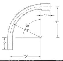
Conforms to UL651 and NEMA TC3 Material is Rigid PVC Bend Tolerance is  $\pm 2^{\circ}$
