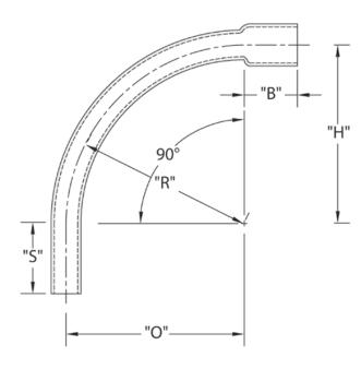
DB-60 Special Radius Bell End 90 Degree Elbows are used to change the direction of a conduit run by 90 degrees.
