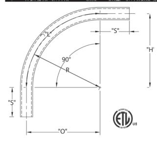
CANTEX Special Radius Plain End Schedule 40 90-Degree Elbows are used to change the direction of a conduit run by 90 degrees when special radiuses are needed.
