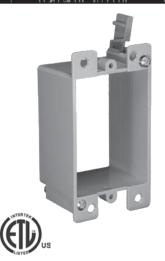
EZ10SOLV is a 1-gang, old work, low voltage EZ BOX used for low voltage installations in renovation (old work) residential and light commercial applications. The backless design is great for the large or deep low-voltage wiring needed for communications and cable installations.
