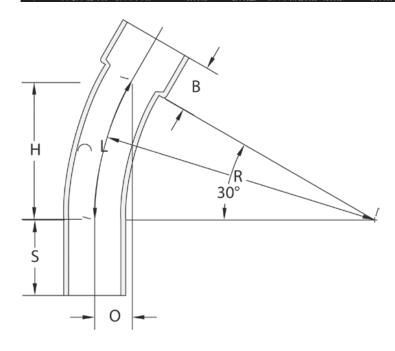
DB-60 Special Radius Bell End 30 Degree Elbows are used to change the direction of a conduit run by 30 degrees.
