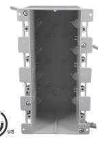
8 V-clamps for EZ & secure wiring EZ68QO EZ BOX is a 4-Gang, 68 cu. in., renovation application (old work) electrical switch or outlet box for residential or light commercial renovation projects when a 4-gang box is needed. EZ mount flanges, winged swing tabs and built in wire clamps make installation easy and cost effective.
