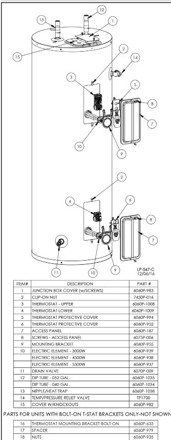
Figure 8 - Replacement Parts - Staged Operation
