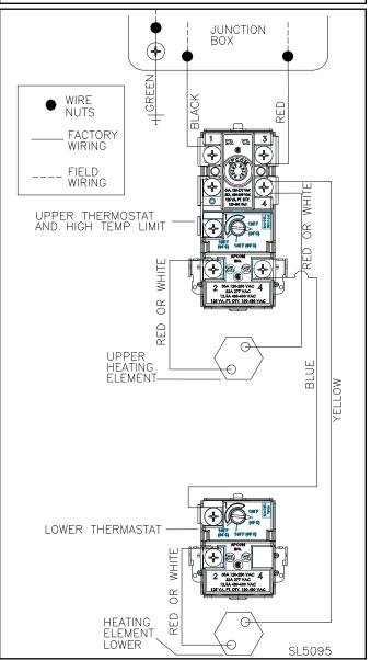
Figure 5 - Dual Element Model Wiring Detail, Staged Element Operation - Green Wire for Grounding the Water Heater
