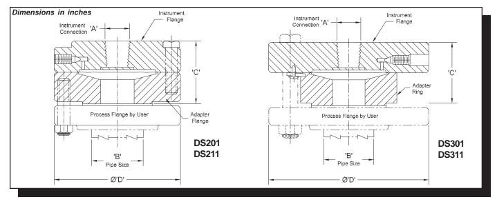
Miljoco flange mounted diaphragm protection seals are ideal for use when the process media of a system will corrode, clog, or otherwise damage a pressure gauge or inhibit its operation. They incorporate a cleanout design, which allows the seal to be disassembled to remove sludge or hardened build-up. A flushing connection is also available so that the system can be piped for continuous flow to prevent media from hardening or caking.
