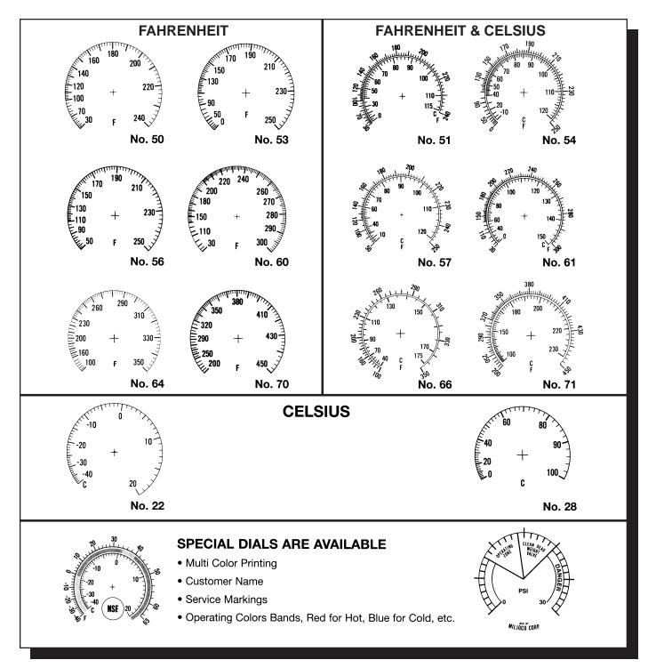
Standard ranges between -40°F and 450°F are offered in single and dual scales. Many are NSF<sup>®</sup> listed for use in food service applications. Vapor actuated thermometers have progressive graduations and are best read in the upper two-thirds of the measuring range, therefore, care should be exercised to select a range that will locate the working temperature in this area. Other ranges and special dials may be available - consult factory.
