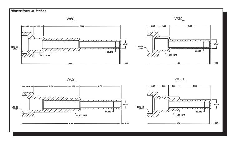
These thermowells are designed for use with Miljoco liquid-in-glass and solar industrial thermometers. They are intended to separate and protect the thermometer from the process or media being measured and allow for the removal of the thermometer without shutting down the process. They are readily available in brass, type 304 stainless steel, or type 316 stainless steel construction to suit a wide range of applications. Other materials are available on request - consult factory.
