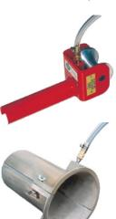
Duct Entry Guide (32500 series): This product fits right into the duct opening and has a roller that the cable must pass over. The unit is fitted with a spray nozzle that when hooked up, places the lubricant right onto the cable as it passes under the nozzle.
