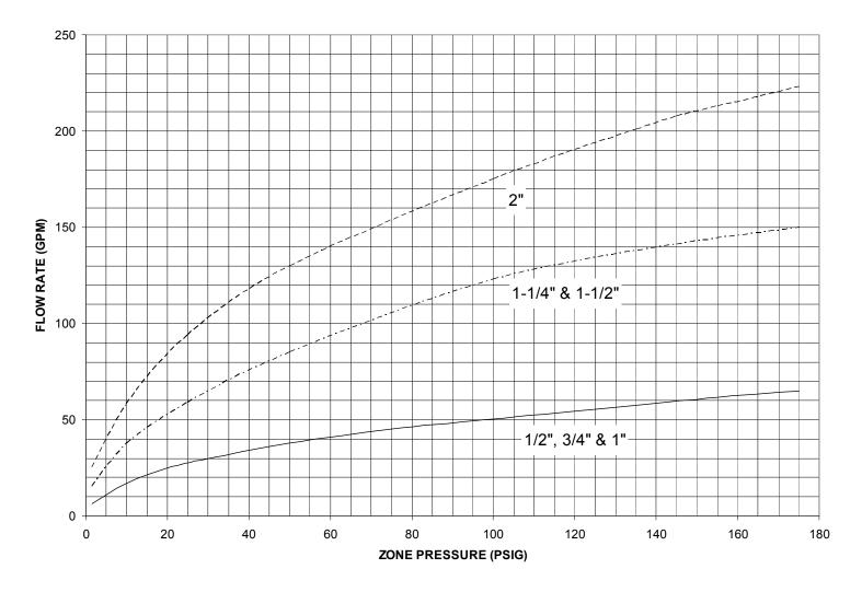
RELIEF VALVE DISCHARGE RATES MODEL RP4A
