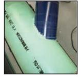
Whether you are cutting a hole for tees or wyes, these guides will keep the pilot bits from "walking", so that you don't ruin the mainline pipe. If you use an Inserta Wye, it is imperative that you cut a teardrop shaped hole.
