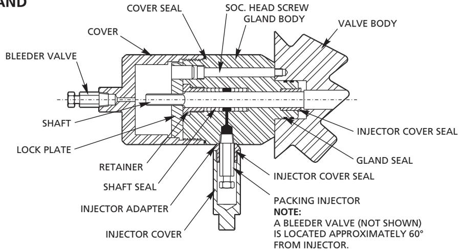
The Type T-Gland is a premium gland for extended shafts on subsea valves. Its' many desirable features include:
