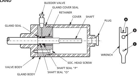
The Type C-Gland is a standard gland for extended shafts on subsea valves. It features a dual seal on the shaft for long trouble-free operation. The shaft is protected by a sealed, screw-on cover. Integrity of the inner shaft seal can be verified using the bleeder valve between the shaft seals. The outer shaft seal can be replaced without disassembly of the valve by removal of the retainer.
