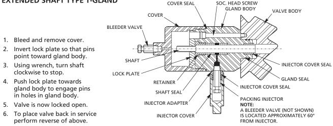
The Type T-Gland is a premium gland for extended shafts on subsea valves. Its' many desirable features include:
