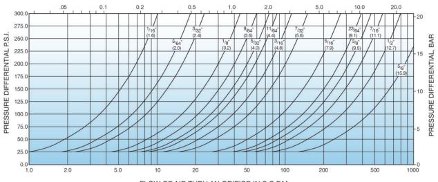
FLOW OF AIR THRU AN ORIFICE IN S.C.F.M. (STANDARD CUBIC FEET OF FREE AIR PER MINUTE)
