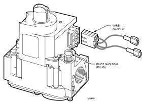
Fig. 8-VR8345 wiring connections in intermittent ignition system.
