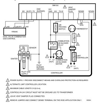
Fig. 9-VR8345 wiring connections in hot surface ignition system.
