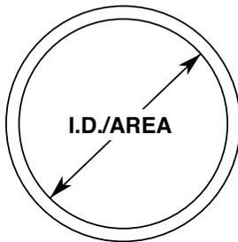
Schedule 5 stainless steel pipe provides larger flow area and greater capacity frequently permitting pipe downsizing.
