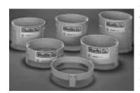
Meter setter box extensions are made from the same material and has the same wall thickness as the shell it will be set on . The lower end of the extension has guides attached to keep the extension properly centered. The top of the extensions are prepared to accept lids as illustrated on page 8F.10\*.
