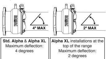
Note: Do not deflect pipe joint after installation.
