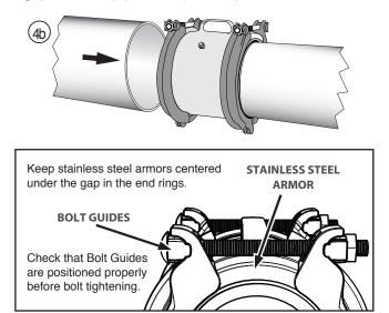
**Step 5** • Tighten each bolt until the gasket contacts the pipe and the coupling is snugly held in place. This should happen at approximately 10 - 20 ft-lbs.
