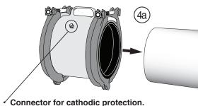
Available as an option. Not included on all MACRO couplings. For more information, contact Romac Industries, Inc. **Step 4b** • Bring the other pipe into position and slide coupling over the gap. There should be a minimum of 2 inches of pipe insertion per coupling end. Confirm proper alignment between pipes and maintain the recommended gap between pipe ends (1/4" - 1/2").
