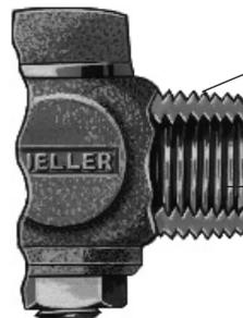
The MUELLER ORI-CORP® Corporation Valve is an easy turning, O-ring sealed, balanced pressure, plug type valve having a round, full open unobstructed flow way. These valves also feature a heavy one-piece bronze body with integral wrench flats.
