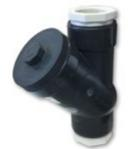
Our ball check valves are made of corrosion resistant PVC and have self-cleaning balls and easy access ports. Available threaded or socket weld for easy gluing to PVC pipe.
