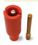
Wire suspension electrodes are designed for use in applications requiring long lengths, or where limited head room prevents installation of solid rod electrodes. Type E-1P shielded electrode is assembled in a molded plastic insulating shield 7/16" in diameter. Type E-1S shielded electrode is assembled in a molded plastic shield 9/16" in diameter.
