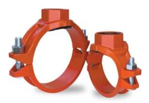
Outlet couplings, sometimes called mechanical tee or saddle tee, allow you to create a mid-pipe branch outlet quickly and easily. A gasket seals on the joined pipe, in the neck of the outlet. The connection is female threaded. These fittings are not recommended for vacuum applications.
