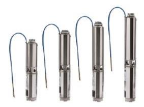
Constructed of high-quality components, these well pumps are designed to be used vertically. A check valve comes standard on all models. If the well pump is positioned in an open body of water, a flow sleeve must be used (p.70)
