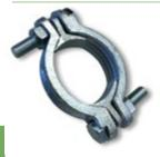
These reusable clamps provide an efficient means to secure fittings for larger size, light or heavy wall hoses. Two-bolt design provides quadruple, full-circumference take-up. Double-tongue saddles bridge the gap between the reinforced, full-width bolt lugs as clamp is tightened, preventing pinching the hose. Can be attached in field or factory with standard tools. Manufactured with plated malleable iron, with steel machine bolts and nuts.
