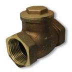
This valve features a screw cap for easy clean out. A hinge-style flapper allows easy low pressure opening and operation. The metal disc makes this suitable for water, oil and gas.
