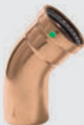
Viega ProPress XL 45° street elbow Smart Connect feature - Copper - Press connection, street components EPDM sealing element Note Must be installed with Viega ProPress XL-C rings and V2 actuator. Model 0926.1XL
