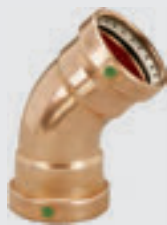
Viega ProPress XL 45° elbow Smart Connect feature - Copper - Press connection components EPDM sealing elements Note Must be installed with Viega ProPress XL-C rings and V2 actuator. Model 0926XL
