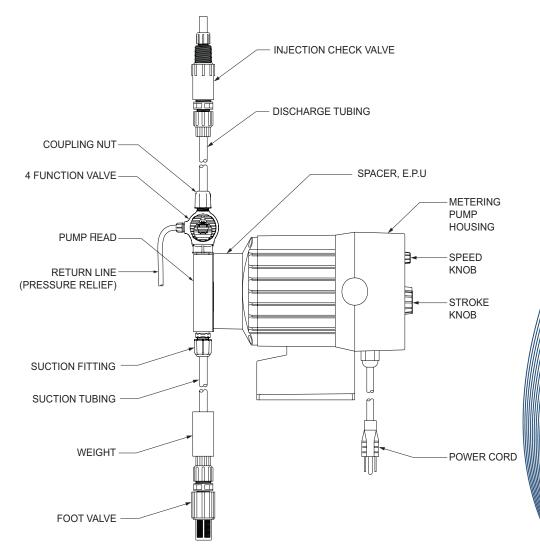
Metering Pump Component Diagram
