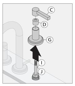
2) Remove cartridge (I or J) from valve body (P) and inspect for debris. Replace cartridge if necessary.
