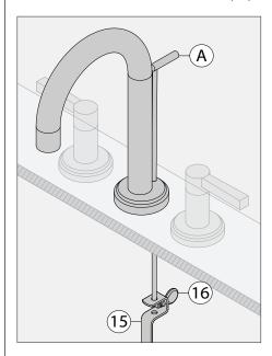
Insert ball rod (11) through spring clip (14) and clevis strap (15).
