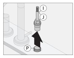
3) Install cartridge (I or J) following the procedure outlined in steps 1 and 2 in reverse.
