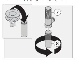
8) Seat flange (2) into sink. From below deck, install gasket (4), washer (5), nut (6) and drain assembly (7) to flange, but **do not** secure nut.
