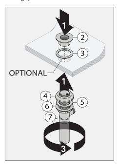
9) Turn drain assembly (7) so rod inlet is facing toward faucet. Secure hardware from below sink. Install stopper (1) in the removable or non-removable position.
