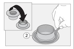
7) Apply plumber tape to threads on tailpiece (8) and install tailpiece to drain body (7), tightening by hand.
