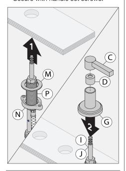
Secure mounting washers (M), mounting brackets (N) and valve bodies (P) to deck surface by tightening mounting screws (O).
