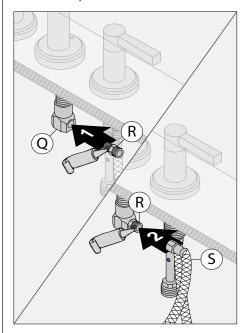
**Note:** Apply pipe sealant to both sides of flex hose adapters (R).
