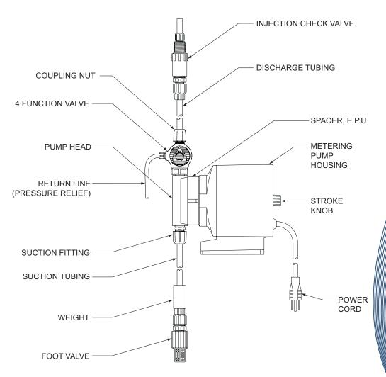
**Metering Pump Component Diagram**
