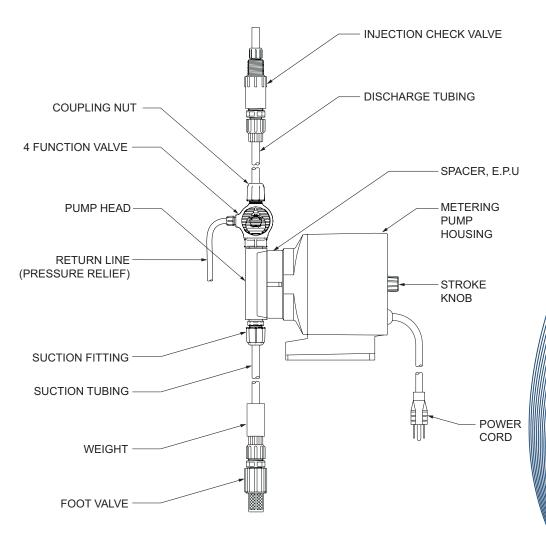
**Metering Pump Component Diagram**
