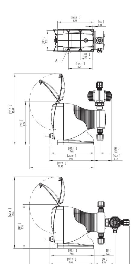
NOTE: ALL DIMENSIONS ARE IN INCHES [MM]. DIMENSIONS SHOWN ARE FOR LARGEST LIQUID END. DIMENSIONS WILL VARY DEPENDING ON LIQUID END SELECTED.
