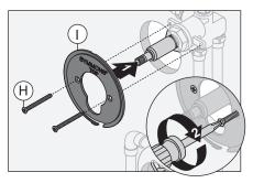
2) Attach diverter escutcheon (G) to mounting plate (I).
