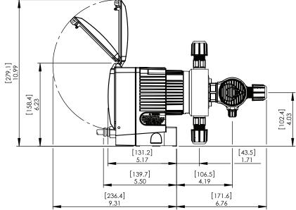
NOTE: ALL DIMENSIONS IN INCHES [MM]. DIMENSIONS SHOWN ARE FOR LARGEST LIQUID END. DIMENSIONS WILL VARY DEPENDING ON LIQUID END SELECTED.
