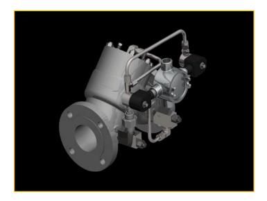
The Model BV 88 Digital Control Valve is designed to provide precise flow rate control and batch delivery of fluid products when used with an electronic batch control device. The Model BV88 features an external pilot control loop that consisits of a normally - open solenoid pilot, a normally - closed solenoid pilot, strainer, and opening/closing speed controls.
