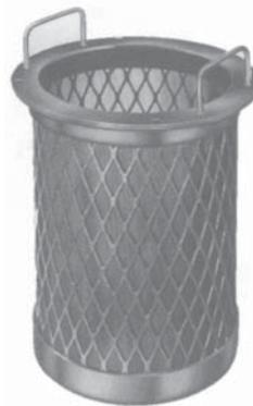
Type of Strainer, Basket used on D-6, D-6-4. Inner screen is soldered to basket frame; may be replaced when required.
