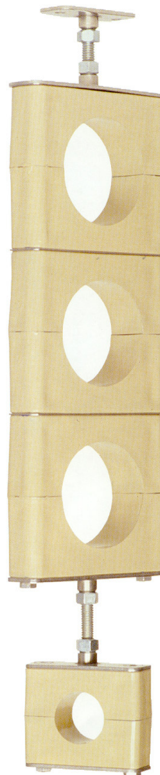
FIG 3: Ceiling mount is the simplest way to suspend pipe or tube while still allowing maximum flexibility in vertical adjustment and pipe direction.
