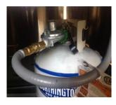
L.P. cylinder is connected to grill via a hand wheel. When full, cylinder weighs nearly 42 pounds to handle with care. Place cylinder in retaining ring and tighten screw on ring to secure tank. Place LP Regulator hand wheel in LP tank outlet, tighten hand wheel.
