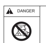
CARBON MONOXIDE HAZARD This appliance produces carbon monoxide which has no odor. Using it in an enclosed space can kill you. Never use this appliance in an enclosed space such as a camper, tent or home.
