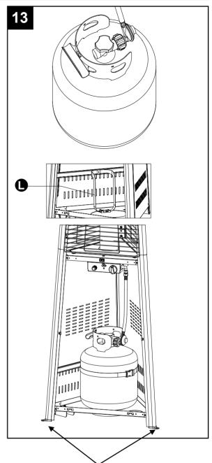
NOTE, we have provided three tabs at the base of the fire feature where it can be secured to a patio. If installed in a windy area or where it may be bumped or tipped (fasteners are not included) we strongly recommend securing *Ambiance* to patio.
